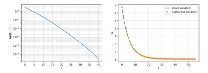
Initial data is an indicator function, e = 0.5 with heat bath  $\tau = 0.1$ . *Left*: Semi-log plot of the relative entropy of f and  $f_{\infty} = f(t = 100, v)$ . *Right*: numerical temperature (orange dots) and exact temperature (blue line). Numerical parameters:  $N_v^2 = 64 \times 64$ ,  $N_\rho = 32$ ,  $M_{\hat{g}} = 16$ , R = 20,  $L = 5(3 + \sqrt{2})$  and  $\Delta t = 0.01$ .
