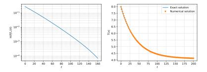
Initial data is a centered reduced Maxwellian, e = 0.95 with heat bath  $\tau = 0.05$ . *Left*: Semi-log plot of the relative entropy of f and  $f_{\infty} = f(t = 100, v)$ . *Right*: numerical temperature (orange dots) and exact temperature (blue line). Numerical parameters.  $N_v^2 = 64 \times 64$ ,  $N_\rho = 32$ ,  $M_{\hat{g}} = 16$ , R = 20,  $L = 5(3 + \sqrt{2})$  and  $\Delta t = 0.01$ .
